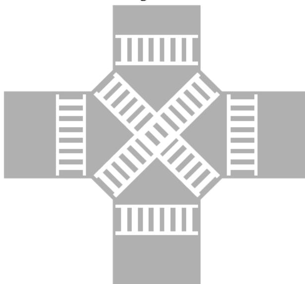
Fig. 7: Ladder pattern at intersection
