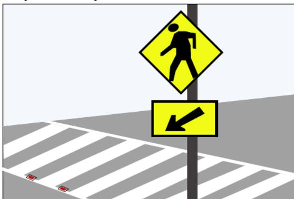
$$\begin{aligned} Gs &= \frac{W}{S_{ped}} + tc(N - 1) + ts \\ &= [(7.5/0.9) + 2(6 - 1) + 3] \\ &= 21.33sec \end{aligned}$$
