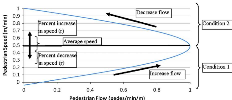
**Fig. 1:** Pedestrian flow—speed diagram used for adjustment factor
